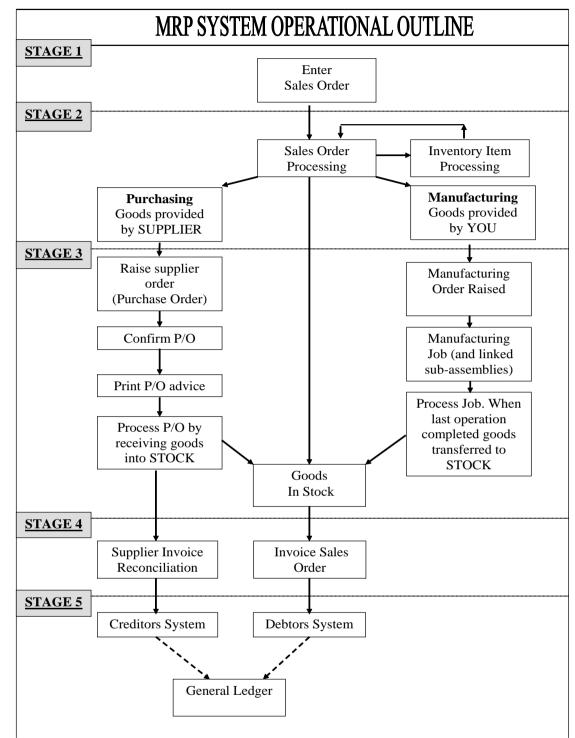
Figure 1- MRP Operation Schematic
